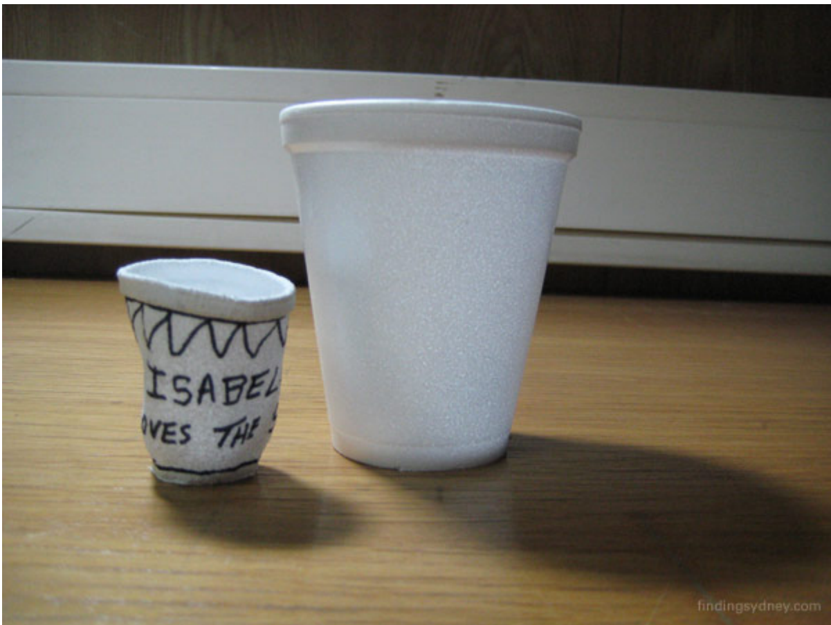
Above Photograph - two polystyrene cups, before and after being squeezed by several thousand metres of water pressure.
